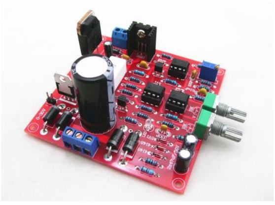
The potentiometer can be installed directly on the board, or with socket and wires. You may also replace it with multiturn potentiometer, which makes adjustment more precise.
