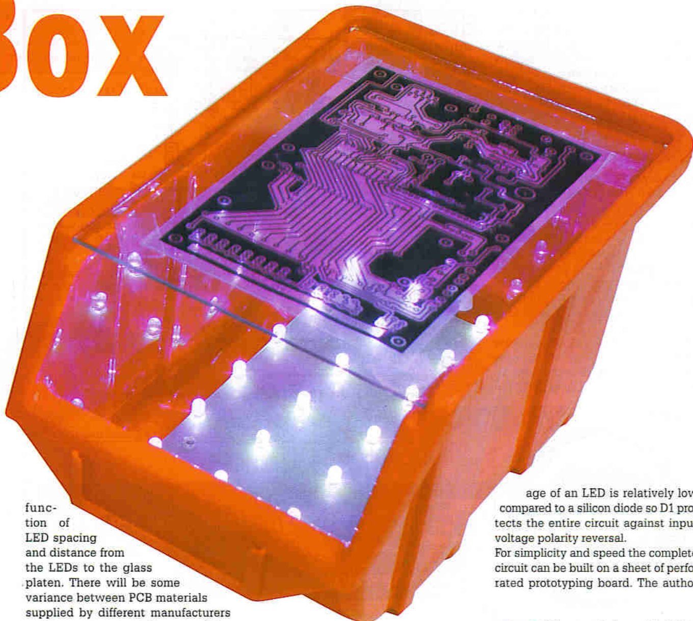
Figure 2. LED layout on the Eurocard sized PCB.
